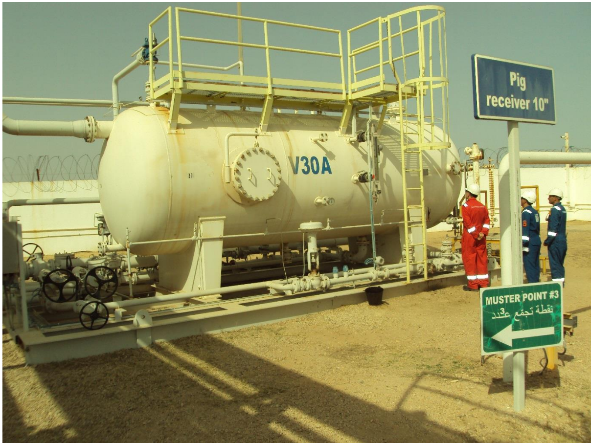
Figure All.12: Pig Receiver
